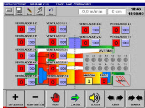
Chamber's blowers control screen
