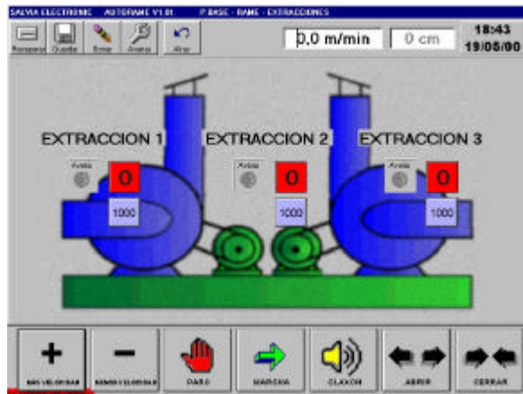
Exhaust fans control screen
