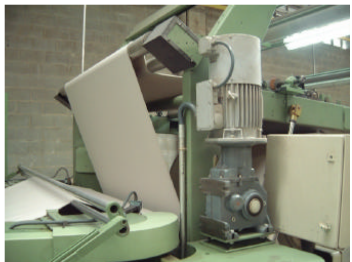
Winding system by charge cell
